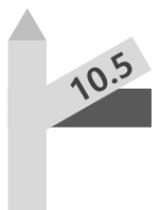
The track inclination is indicated by signs of this type on the side of the rail. The
