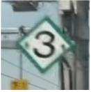
This number indicates the stop position for a train with as many cars (or fewer) than the number displayed. You therefore need to know the number of cars in your train (indicated on the simulation settings screen).
