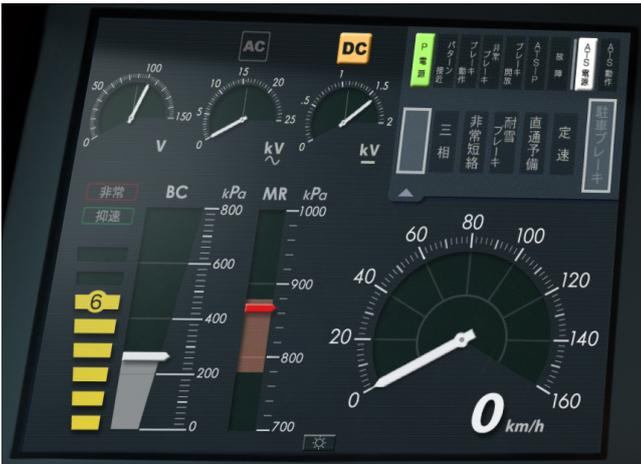
The first screen (train technical info) displays electrical voltages (including DC/AC indicator) and various indicators at the top.
