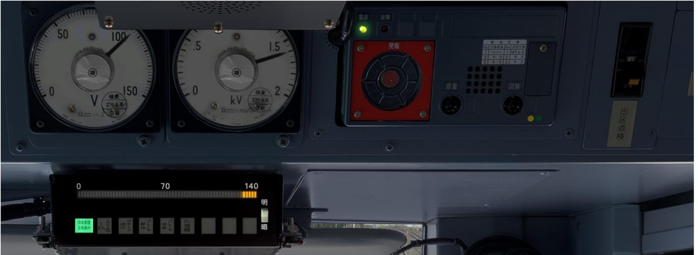
The upper part contains the electrical voltage indicators, the ATS-P dial, the train protection radio equipment and a few other buttons.
