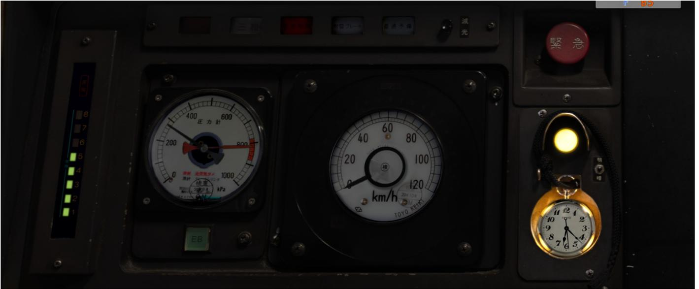
On the left is the brake level, with the emergency brake indicator "□□".
