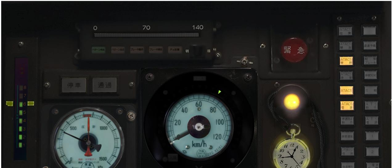
On the far left, we have the brake levels, with a yellow line on level 6 to indicate the level to apply when stopping and indicator for emergency brake in red (□□ ).
