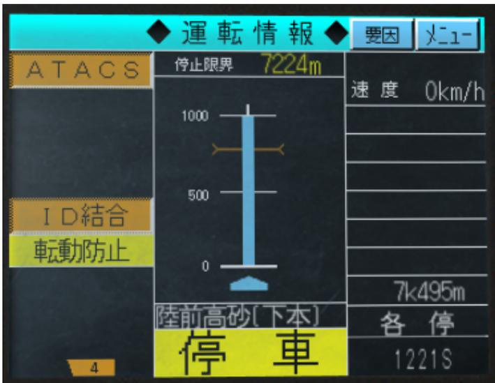
The single screen contains some information about the line, when you're on the section using ATACS.
