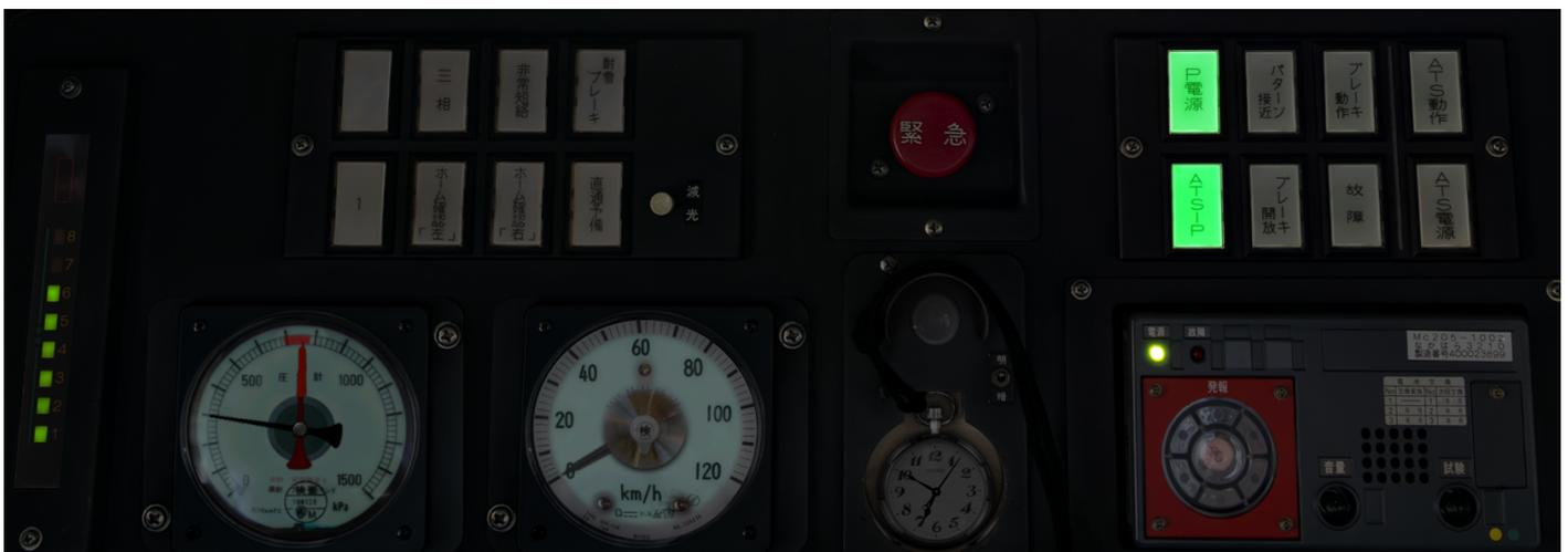
On the far left, we have the brake levels with an indicator for emergency brake in red (緊急).
