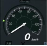
For trains using the D-ATC (Digital Automatic Train Control) or ATACS (Advanced Train Administration and Communications System) safety system, the maximum speed is represented by a green arrow on the speed dial. This applies to the Keihin-Tohoku and Yamanote lines, among others.
