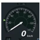
For trains using the D-ATC safety system, maximum speed is represented by a green arrow on the speed dial. If the maximum speed is exceeded, the train will automatically brake more or less hard to go below the limit.
